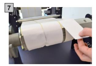
Temporarily attach the label directly to the take-up core holder.
