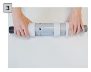
Insert the empty cardboard cores on the core holder to receive the new labels roll.
