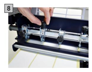
Position the blades in between each column and on either edge if desired.
