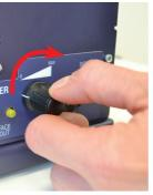
Switch on the unit and slowly increase the speed up to the requested working speed.
