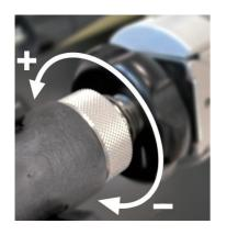
It is possible to adjust the clutch by just screwing or loosening the aluminium handle on it.
