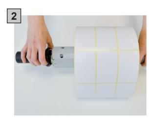
Tighten the roll and the guide in place by turning the tension knob.
