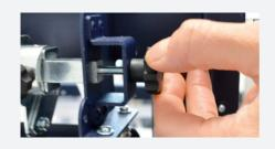
The black knobs lock the slitter module in the requested position. Screw the thumb knobs to move the blades to the right or to the left.
