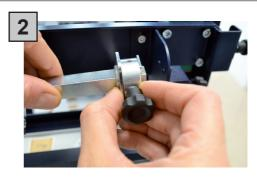
Slide in or out the blade holder. Relocate the slide iron bar in its position and rescrew the thumb screw.
