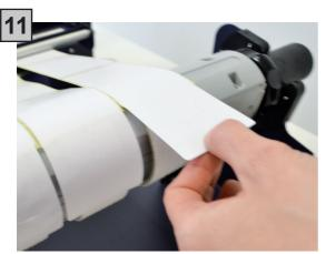
Attach the labels to the core using waste label or tape.
