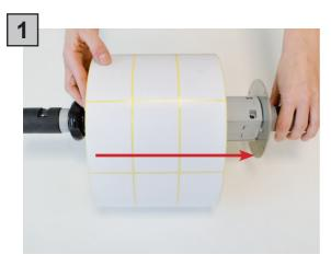
Load the roll on the core holder. Push until it touches roll guide.
