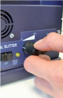
Slowly turn the speed knob. Run the SLITTER until the slit labels reach the bottom of the take-up core holder.
