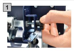
Keep out the iron slide bar unscrewing the thumb screw.
