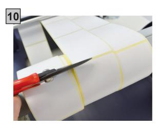
Remove the labels that have wrapped around the take-up core holder.
