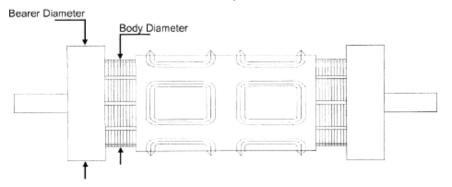
Mirror-finish tight-tolerance magnetic cylinder: Difference of body and bearer diameters held to +.0000/-.0001"(2.5 microns).
