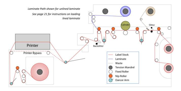
Load the unwinder with the desired media. Follow the path shown above, either through the printer for in-line operation or using the Printer Bypass path to cut blanks or pre-printed stock.
