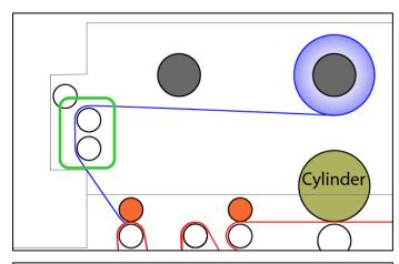
Laminate Path for lined laminate
